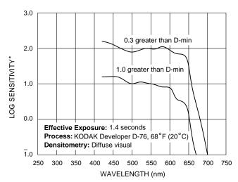
\*Sensitivity = reciprocal of exposure (ergs/cm²) required F002\_0523AC to produce specified density
