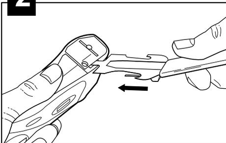
Insert tool into film door slot.
