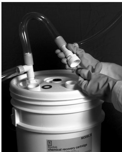
Remove the washers from the caps of the new cartridge.
