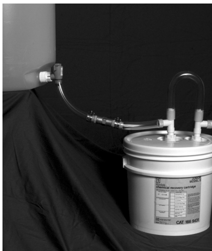
A KODAK Chemical Recovery Cartridge being fed from a raised holding tank. Place the tank outlet slightly higher than the inlet of the circulating unit as shown.
