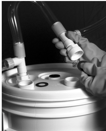
The circulating unit directs the flow of solution into and out of the cartridge, and provides a bypass in case of blockage in the cartridge.
