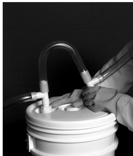
Press down firmly to pump out the solution in the circulating unit.
