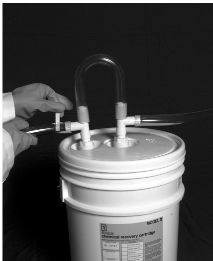
In this illustration, the desilvered solution is being tested with a silver estimating test paper.
