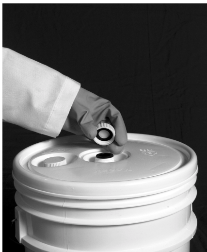
Remove the plastic caps from the new cartridge.
