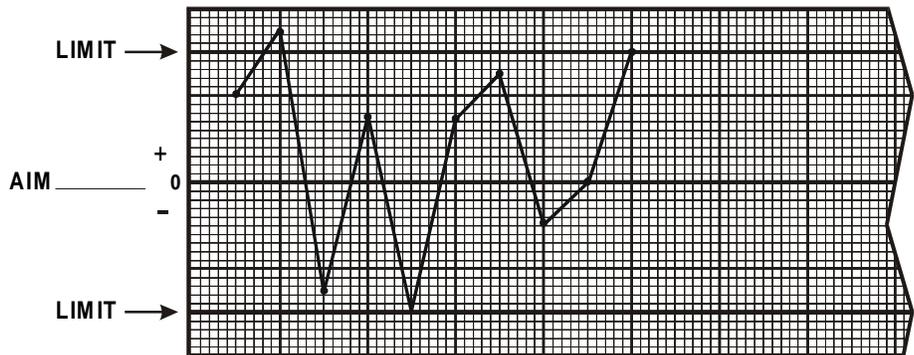
Variability is unacceptable, and the process is not on aim. Variability must be reduced first, and then an adjustment is required to move the process to the aim.
