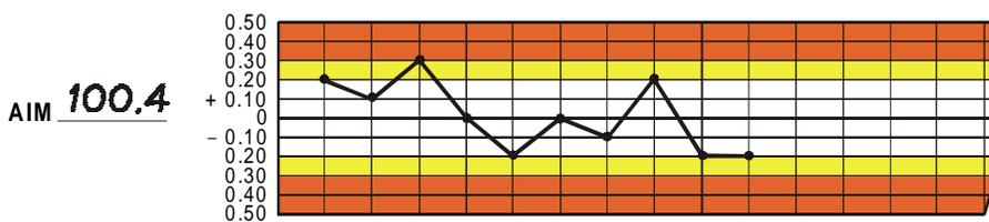
The variability in the process is acceptable, but the process is not on aim. An adjustment is required to center the process on aim.
