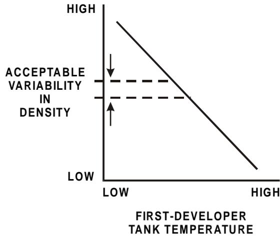
The tolerances (control limits) for first-developer temperature are determined from the acceptable level of density variability in the processed film. Note that the tolerances are narrow to maintain tight control of density.
