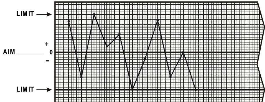
These examples show that simply being within the tolerances is **not** enough. The process must be controlled to the aim **and** have minimum variability.
