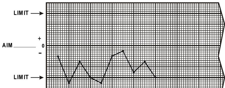
The process is in control for variability and is on aim. The data points are centered on the aim, and at least 7 out of 10 points plot within the third of the tolerance range immediately above or below the aim.
