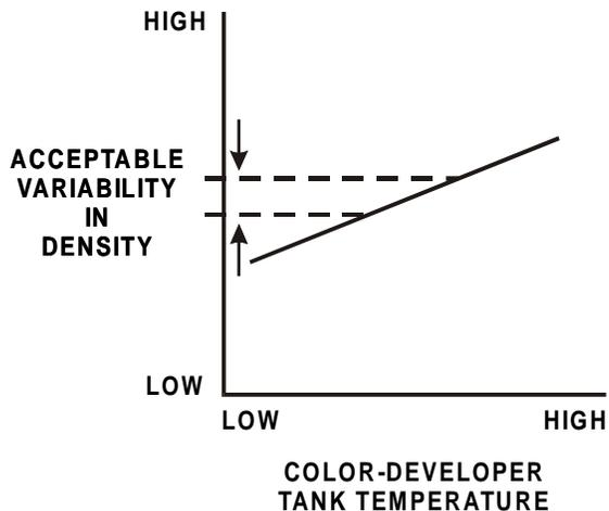
Tolerances for color-developer temperature are determined from the acceptable level of density variability in the same way that they are for first-developer temperature.
