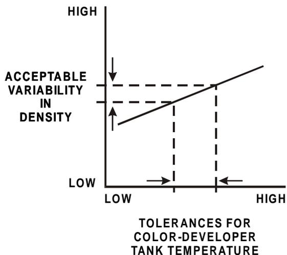
The aim for a process parameter is centered within the tolerances, as shown here for first-developer temperature:
