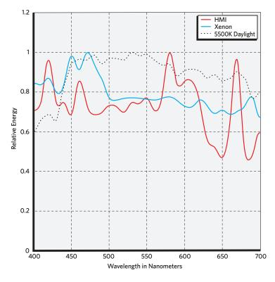
Relative spectral energy curves for the HMI and Xenon lamps compared to the 5500K Daylight curve.
