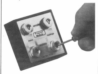
The Program is now entered into the module and will remain there until the Module Controls are reset. Verification numbers should be entered in pencil on the eraseable spaces on the module faceplate (see following section, PROGRAM VERIFICATION).
